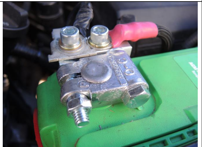
Detail of Positive Battery Post with optional parts ( Step 6A )
