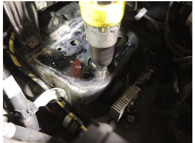
Drill / enlarge four holes for M8 Riv Nut ( Step 2B )
