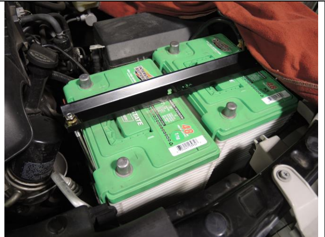
Dual battery Tie Down installed ( Step 5B )
