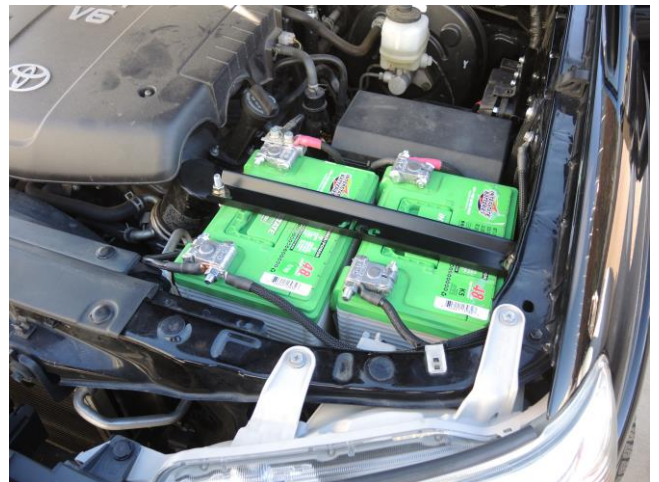
Completed dual battery installation ( Step 6D )
