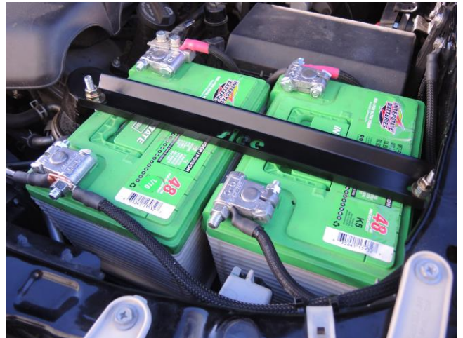
Completed dual battery installation ( Step 6C )
