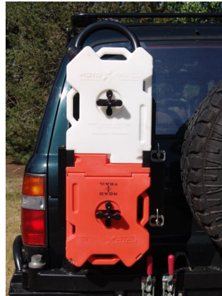
Installation completed with Rotopax ( Step 5 )
