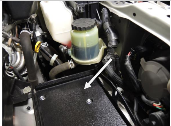
ABS riser installed (Step 6)
