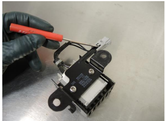
Remove connector from bracket ( Step 2B )
