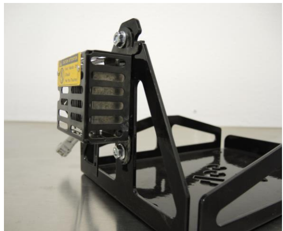
Mount DRL resistor to Slee tray ( Step 2C )
