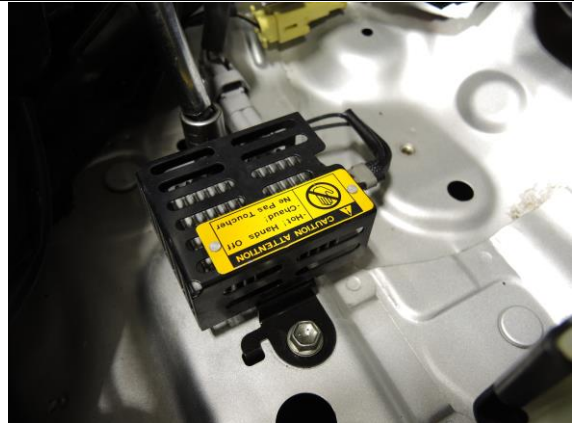
Remove bolts and unplug harness ( Step 2A )
