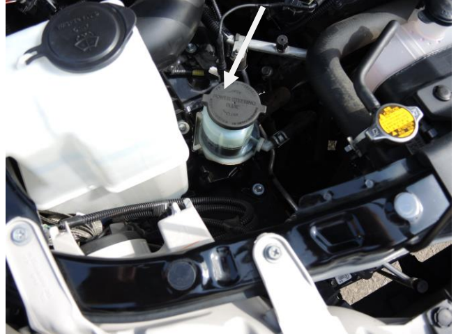
Location of Power Steering Reservoir ( step 2 )
