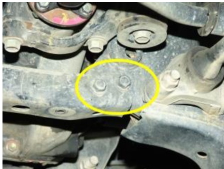
Side bolts of the existing cross member
