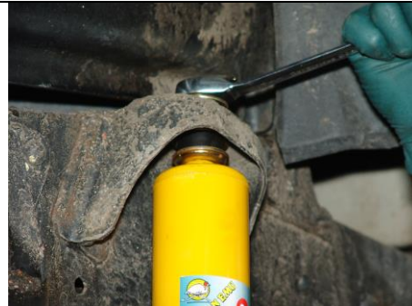
OME Shock installation (Step 24)
