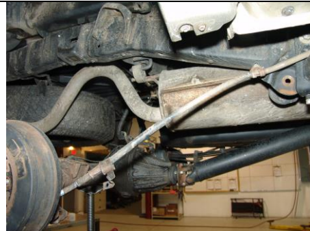
Rear leaf spring removed (Step 17)
