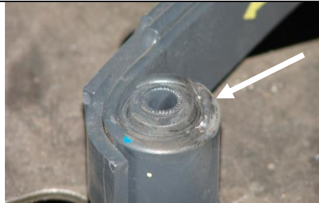
Weld bushing (Step 20)
