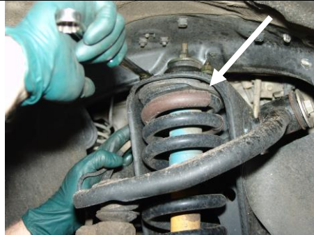
Don't remove center nut ( Step 7 )
