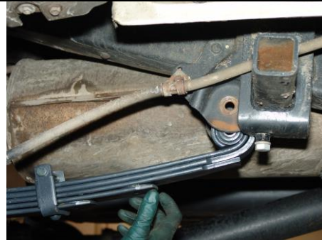
Install Leaf Spring (Step 22)
