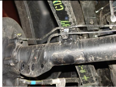
Remove U bolts (Step 16)
