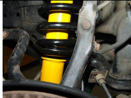
Coil spring and strut assembly installed ( Step 13 )
