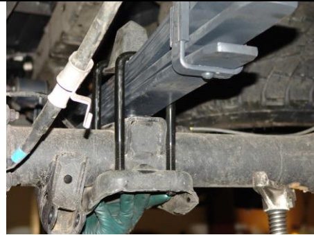
Install U bolts (Step 23)
