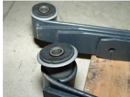
Bushings installed in background in process in foreground (Step 19B)
