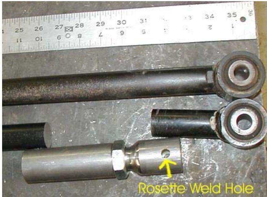
1. Remove oem panhard rod from vehicle and mark the end that was attached to the frame.
