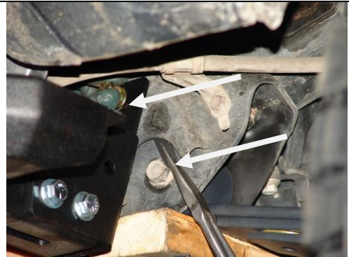
Install Bolt (Step 9)
