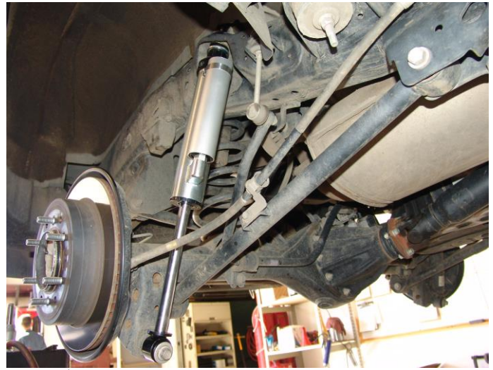
5 th Gen 4Runner - Rear shock orientation (Step 4)
