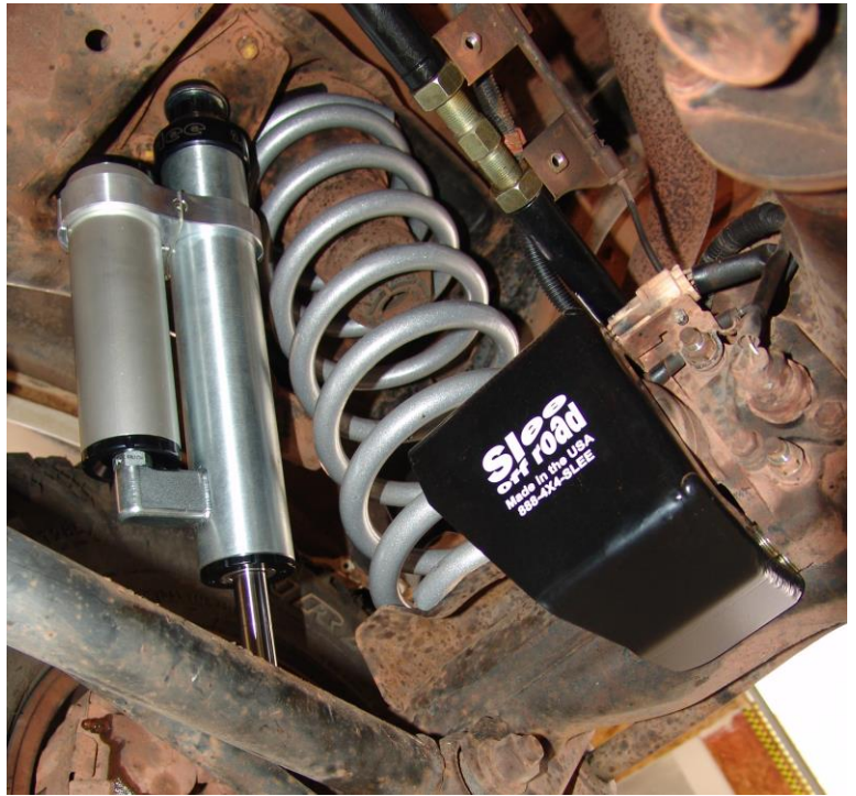
80 Series - Rear shock orientation (step 2C)
