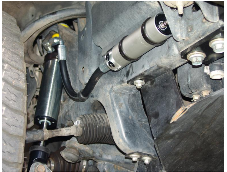
100 Series – Front shock orientation ( step 3A )
