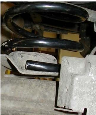
**Rear spring installed and end of coil seated properly.**
