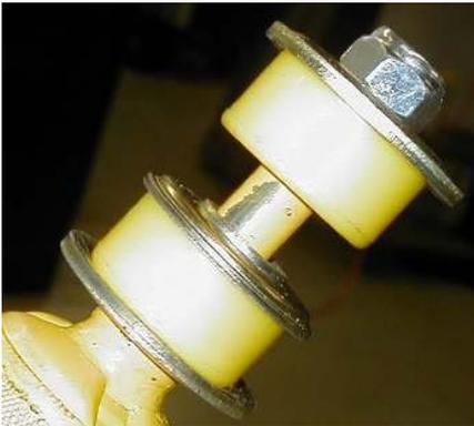
**Bushings and washers installed on shock stem. The order is important. Note the indexing washer that is installed in the middle. This is the washer with the lip on it. This lip is to locate the stem in the shock mount hole. Note: the bushings are installed on the pin for illustration purposes only. The nut, first washer and first bushing will not be in position when the shock is installed.**
