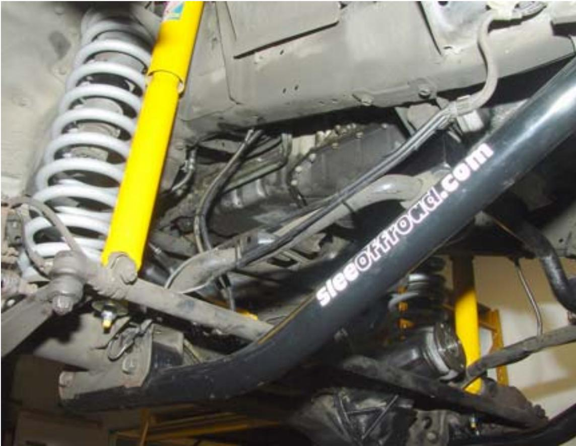
Front control arms installed. This photo shows the ABS lines modified and attached to the swaybar.
