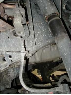
**Passenger side brake line bolts removed.**
