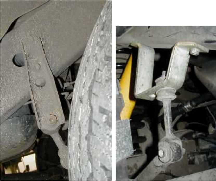
**Photos showing the two different swaybar mounts that were used on the '91-'97 Land Cruiser**
