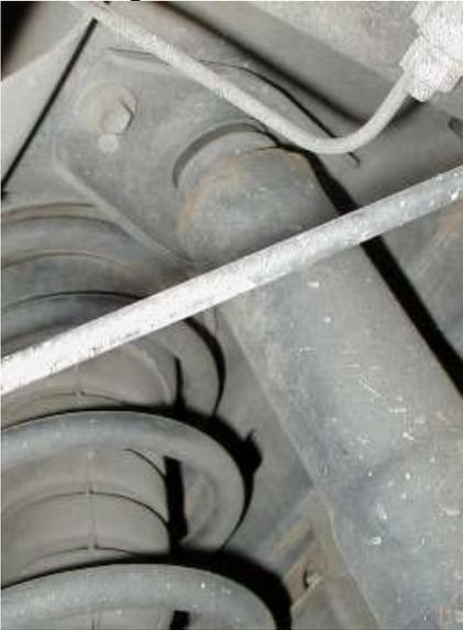
**Top shock mount plate showing one bolt. There are two bolts. One each side. The heads are 14mm. These bolts are removed and then the shock is removed with the plate still attached. Do not mix the PS and DS plates. They are side specific.**
