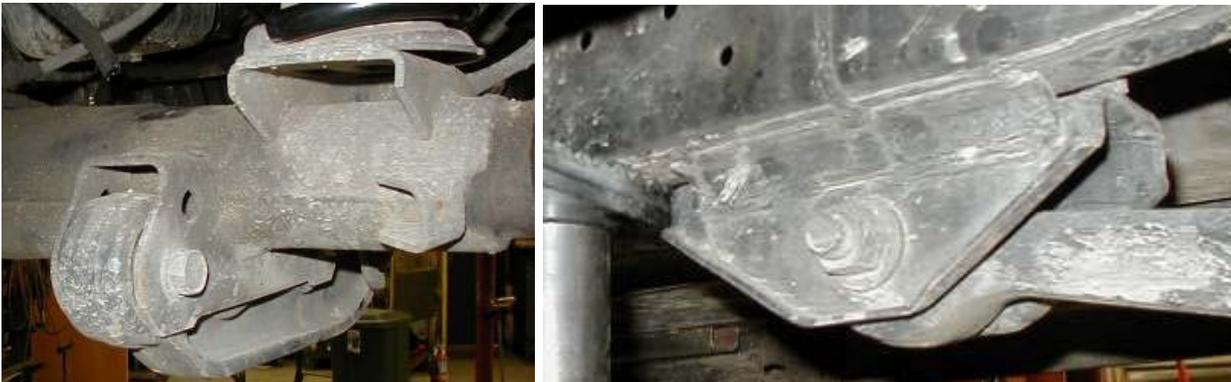
**Front control arm mounting bolts.** These bolts are removed by loosening the bolt and not the nut. The nuts have serrations on the face and it locks in place.
