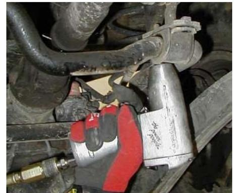
**Removing the front swaybar bracket bolts.**
