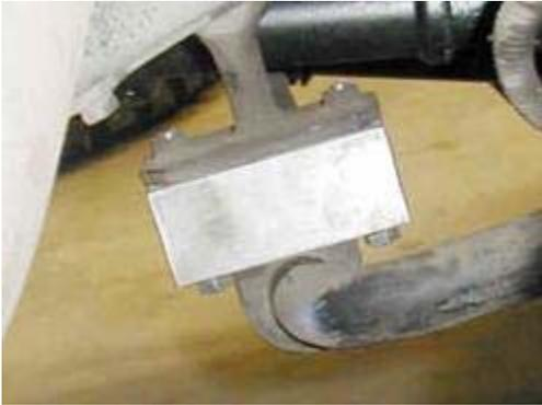
**Swaybar block installed on front swaybar.**
