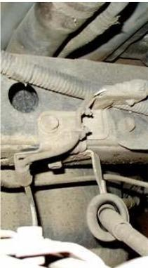
**Rear brake line bracket and emergency brake cable guide still attached to the frame.**
