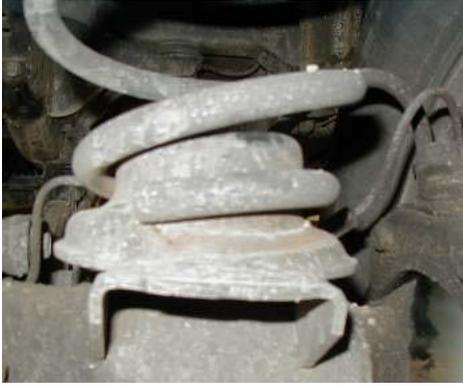
**Driver side spring unloaded. Not the position of the end of the coil. Make sure the new springs are installed with the end of the coils in the proper location.**
