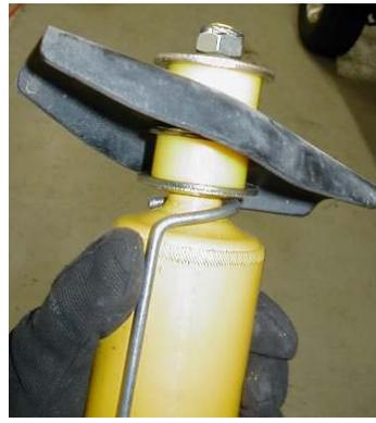
**Rear shock installed on mounting plate prior to tightening the shock nut.**
