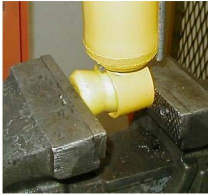
**Pressing the bushing into the eye on the rear shocks using a vice.**
