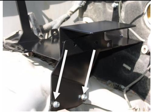
Install support Bracket (Step 6)
