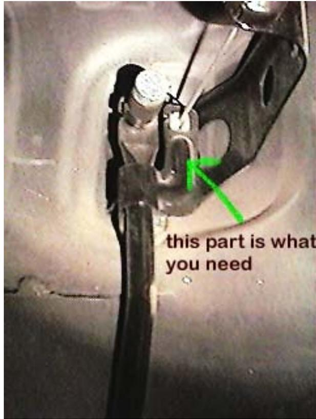
**Photo of upper part of the gas pedal. The J shaped bracket has to be present. If this is not, you would need to replace the gas pedal with a later model one.**
