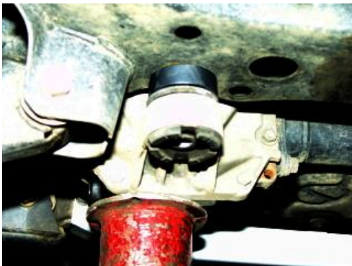
New Slee Cross Member bracket installed ( Step 7 )
