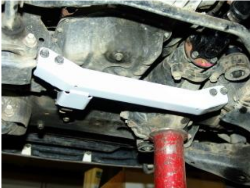
New Slee Cross Member bracket installed ( Step 7 )
