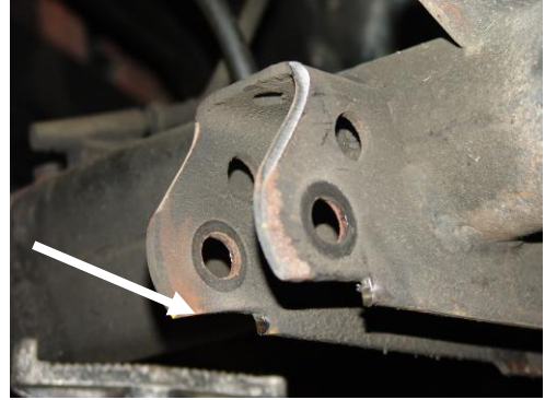
Control arm axle bracket shown cut (Step 4A)
