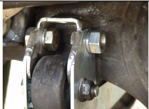
Passenger side Caster Plate shown (Step 5A)
