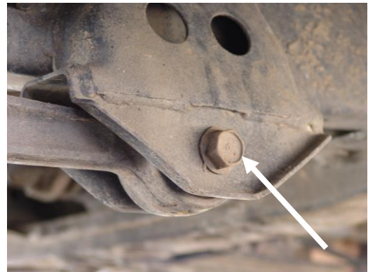
Loosen bolts at frame (Step 2B)
