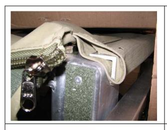
3. Remove alu angle section and slide it into awning sleeve marked TOP, centralise awning, push a hole through canvas material with a sharp object or use soldering iron. Fit and tighten awning bag together with alu angle section with M6 x 20 bolts, washers and nuts.
