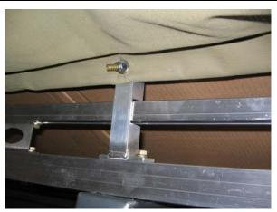
5. Position and fit T bracket in the centre of the awning. Drill 8.5mm hole through angle section and awning bag sleeve. Fit M8 x 40 bolt from inside out. This 8mm bolt is used to locate the fibreglass rod which holds up the centre of the awning.
