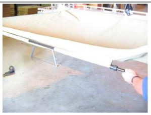
6. Unroll awning. Slide in adjustable front rod. Push rod into both arms, extend rod on both sides and tighten up on plastic nuts.
