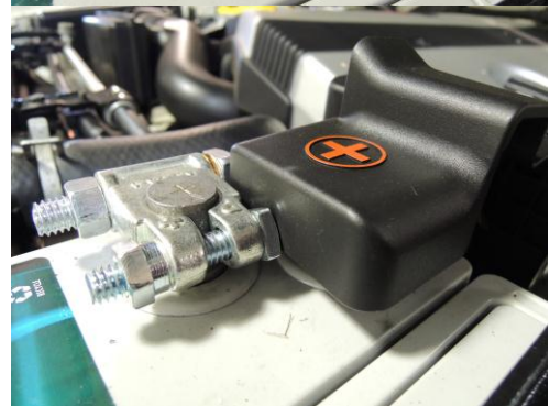
Install posts and connect battery ( Step 7 )
