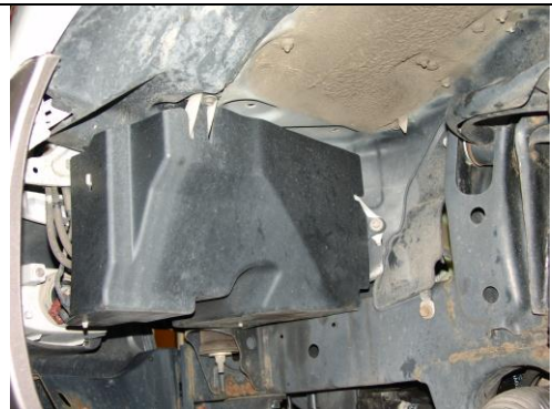
Remove hardware on reservoir ( Step 2 )
