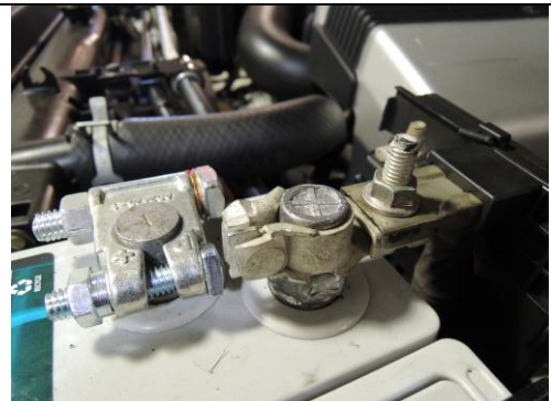
Double Nut on J-Bolt (Step 5B)
