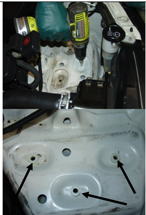
Drill and install spacers ( Step 3 )
