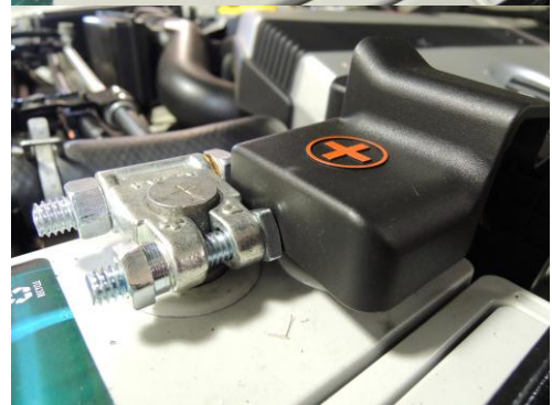
Install posts and connect battery (Step 7)
