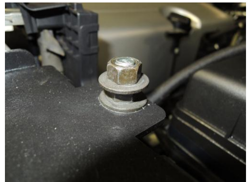
Double Nut on J-Bolt ( Step 5B )
