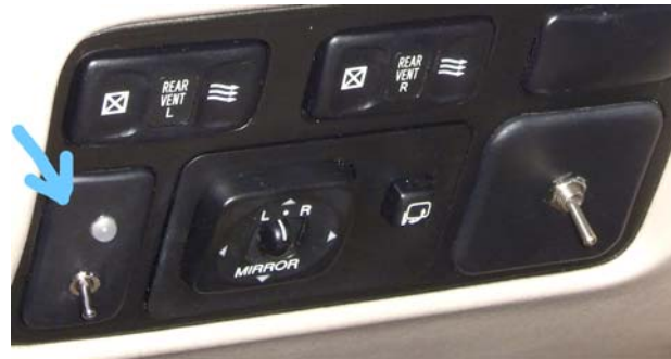
Height Control unit fitted to switch blank-off plate (Installation photo's courtesy of Vic Bentley)
