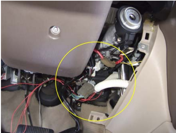
Location of AHC Unit
