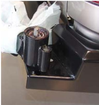
**Tire Carrier installed on bumper.**
