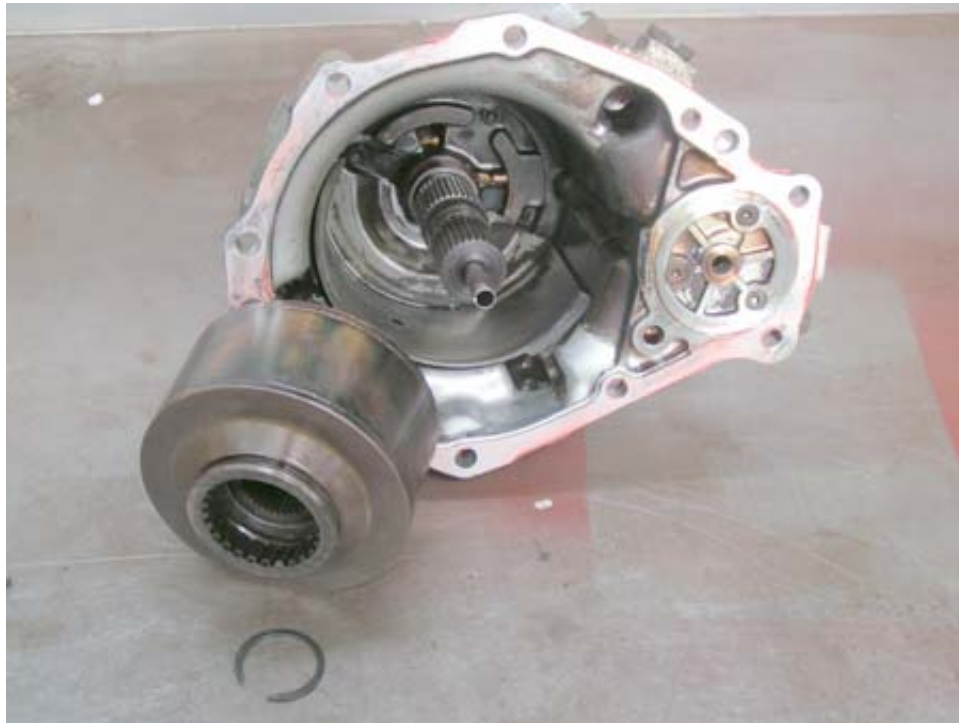
The photo below shows the viscous coupling removed from the extension housing.
