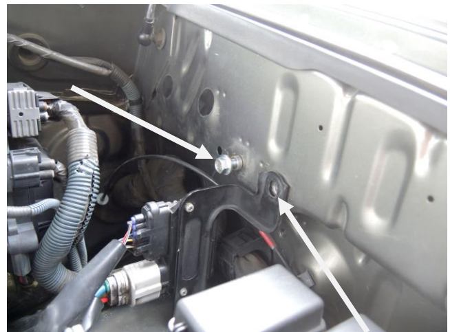
Remove bolt from bracket, install bolt with spacer – do not tighten ( step 5A )
