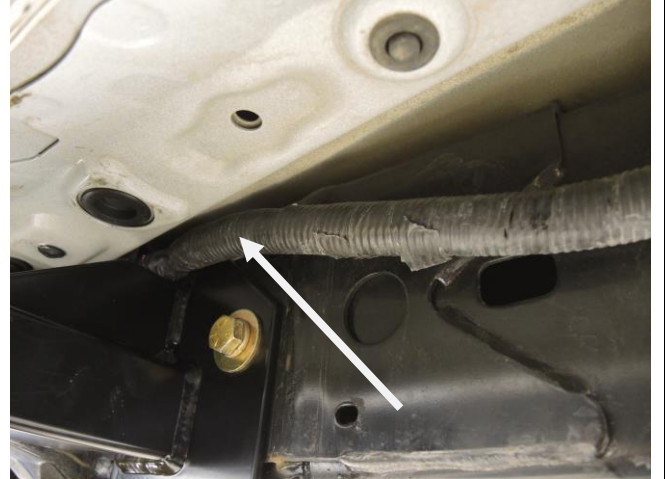
Install Driver side Slider - verify wiring harness has clearance (Step 7A)
