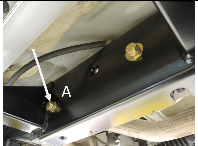
Begin installing passenger slider ( Step 3A )
