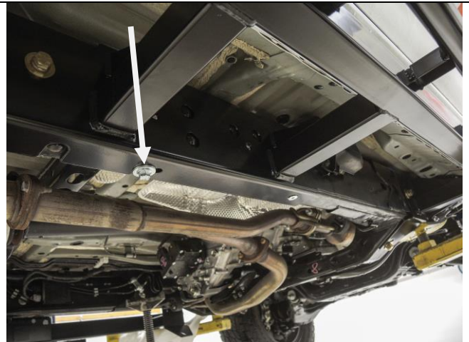
Install bolt removed in Step 2 (Step 6)
