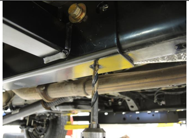
Drill two holes to 3/8" (Step 5B)
