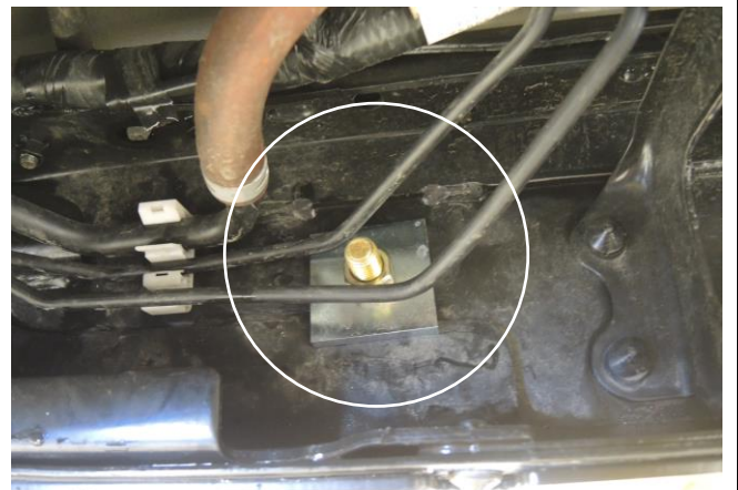
Verify brake line clearances (Step 7C)
