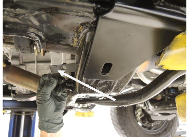
Install 'Z' Shaped Nut plate and 1/2" Bolt, lock washer and washer ( Step 4C )
