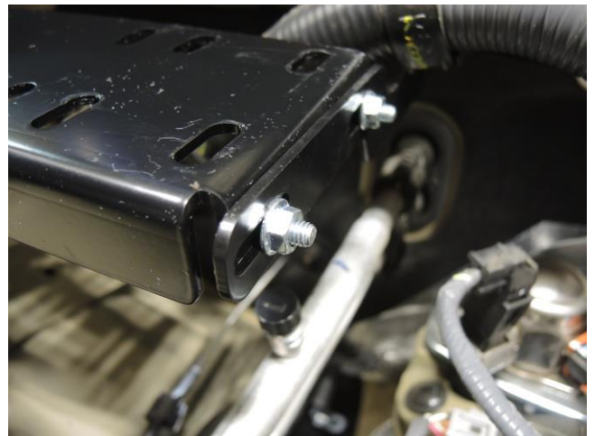
Bolt orientation for Twin Compressor (Step 1C)
