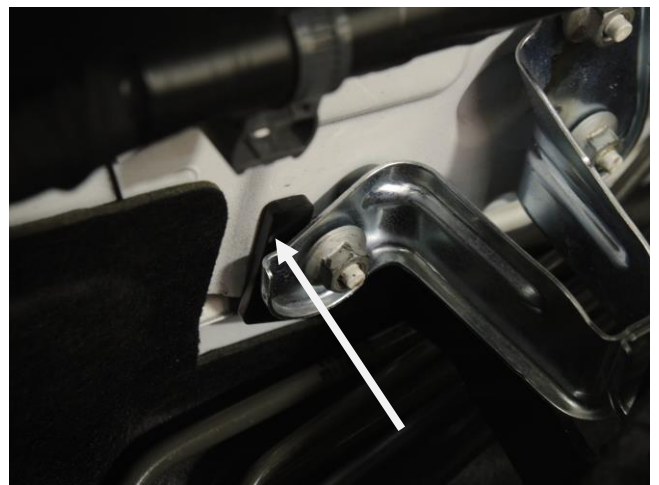
Leg support orientation to firewall ( Step 4C )
