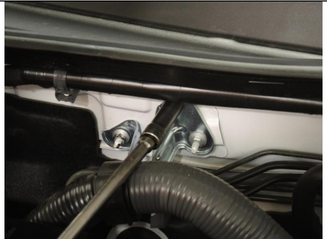
Loosen three nuts at firewall, install leg support ( Step 4A )
