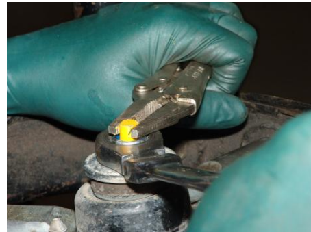
Tightening top strut nut ( Step 10A )
