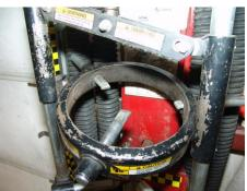
Wall Mounted Strut Compressor (Step 7)
