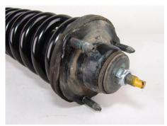
View of assembled strut top (Step 10B)
