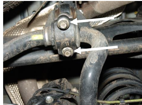
Remove sway bar bolts ( Step 14A )
