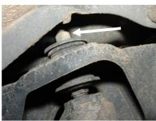
Remove rear shock top nut (Step 15A)
