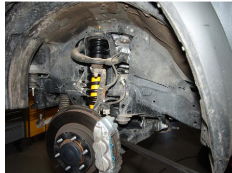
Coil spring and strut assembly installed ( Step 11 )
