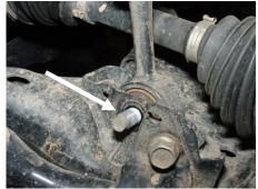
Lower shock nut and washer removed (Step 5)
