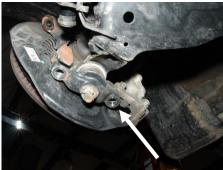
Two ball joint bolts removed (Step 4)
