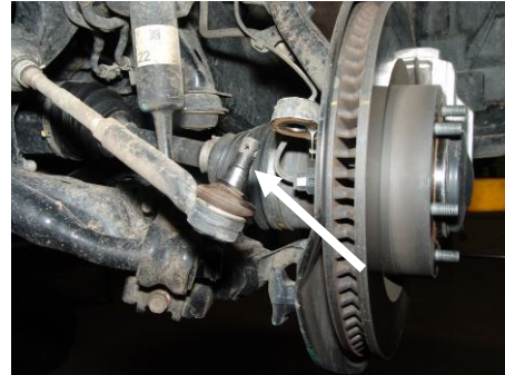
Ball Joint removed (Step 2)
