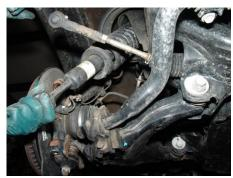
Removing strut assembly (Step 6)
