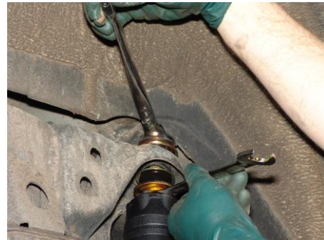
Tightening top nut of shock (Step 19A)
