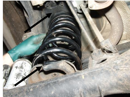
Spring seated correctly (Step 18B)
