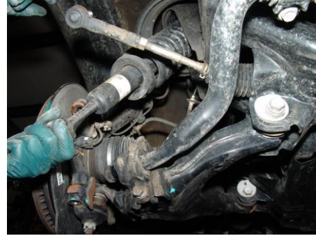
Removing strut assembly (Step 6)
