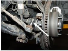
Ball Joint removed (Step 2)
