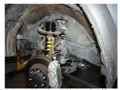
Coil spring and strut assembly installed (Step 11)
