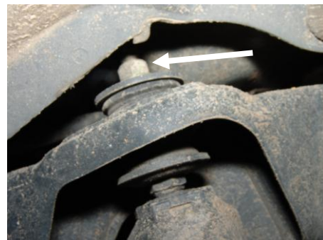
Remove rear shock top nut ( Step 15A )
