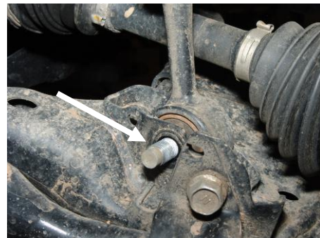
Lower shock nut and washer removed (Step 5)
