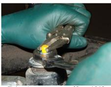
Tightening top strut nut (Step 10A)
