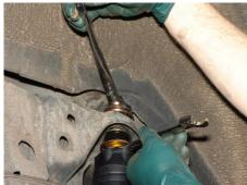
Tightening top nut of shock (Step19A)
