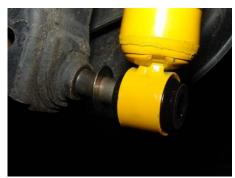
Installing shock (Step 19B)
