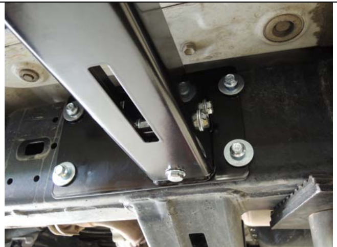
Front Frame Leg shown (Step 7A)
