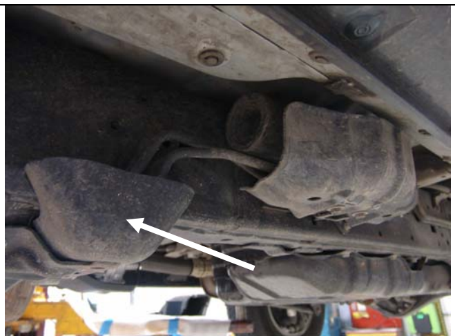
Remove two KDSS cover (Step 8A)
