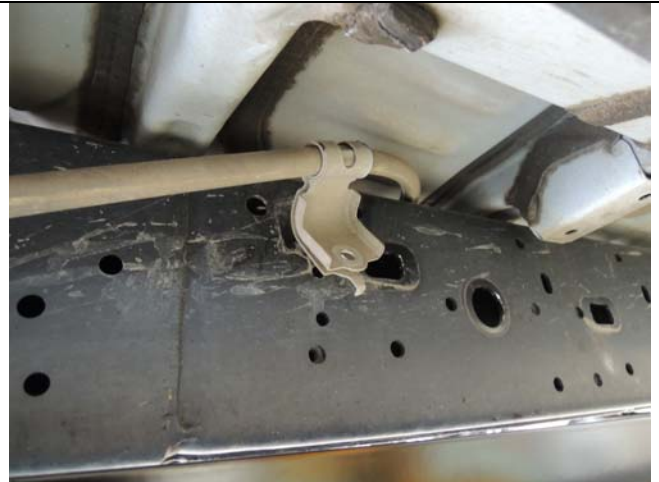
Remove parking brake cable attached to frame (Step 4)
