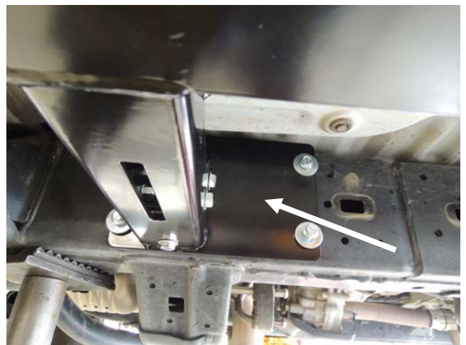
Front Frame Leg Bracket (Step 8B)
