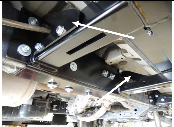
Support legs installed (Step 7C)
