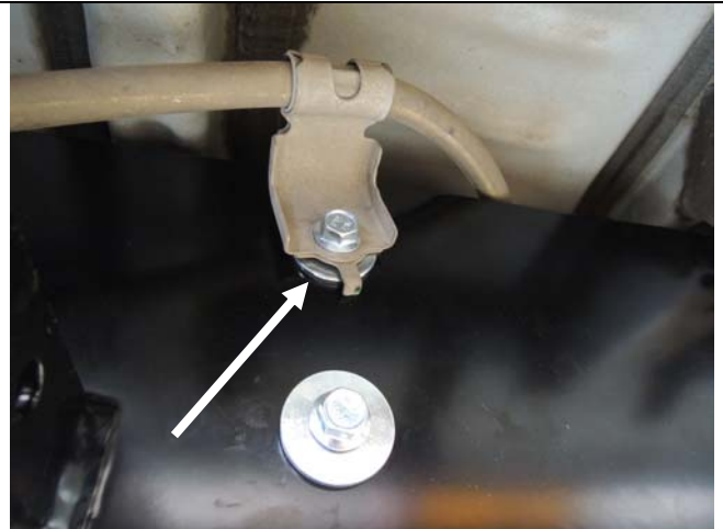
Support fuel tank – remove bolt on strap (Step 10B)
