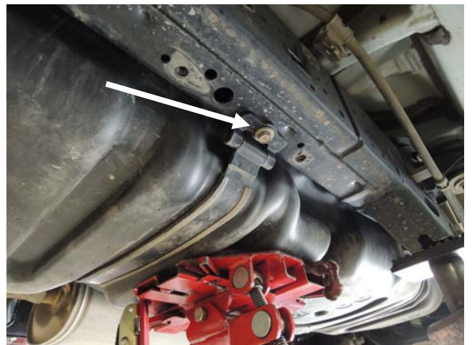
Support fuel tank – remove bolt on strap (Step 9B)
