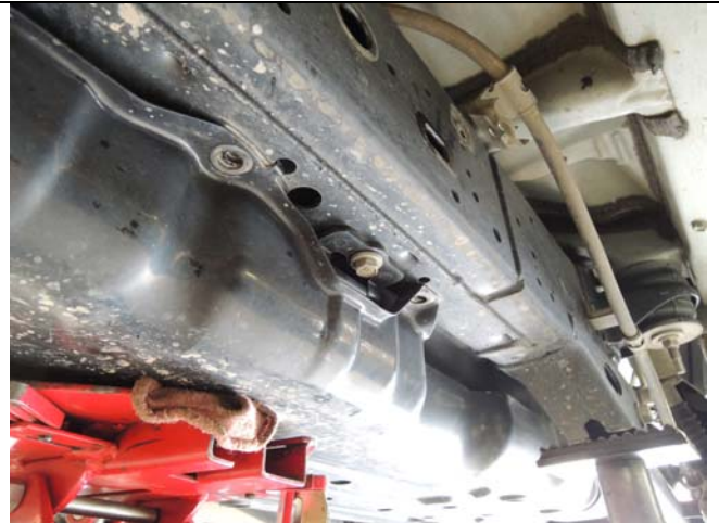
Support fuel tank – remove splash pan (Step 9A)
