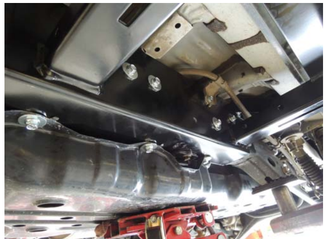
Detailed view of fuel tank strap and splash pan (Step 10C)
