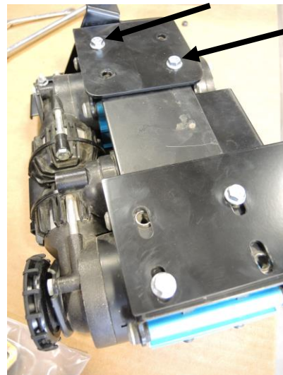
Mount compressor to bracket ( step 7 )
