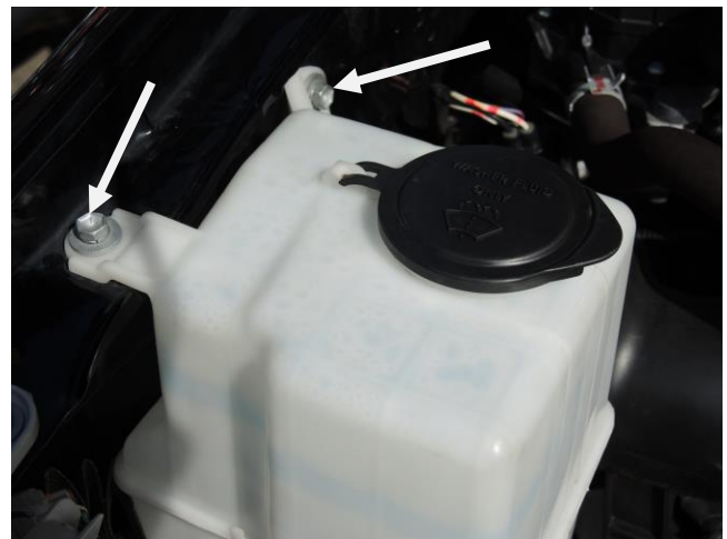
Remove Washer Fluid Reservoir ( step 3 )
