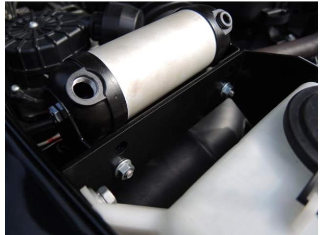
ARB Manifold Kit Installed for reference ( step 13 )
