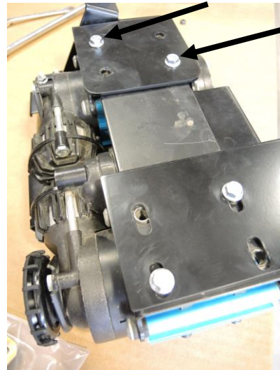
Mount compressor to bracket ( step 7 )
