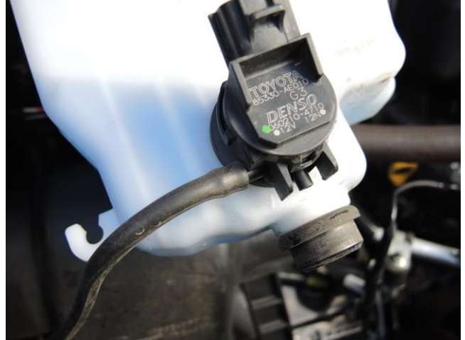
Plug hose disconnected to prevent loss of fluid ( step 3B )
