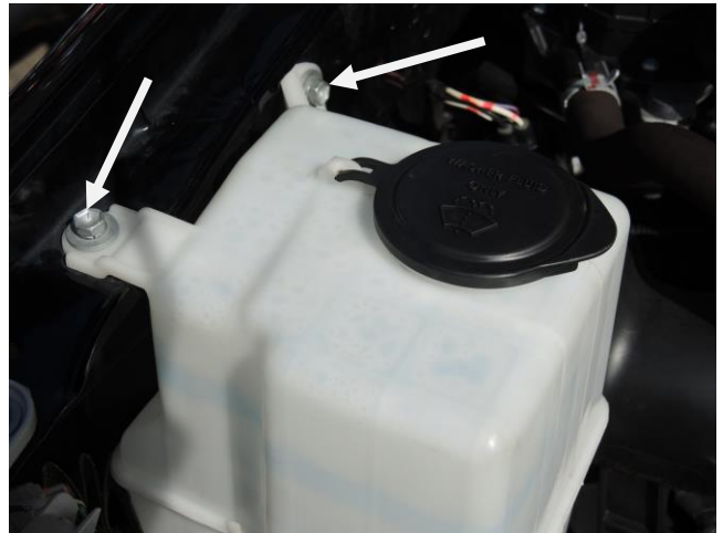
Remove Washer Fluid Reservoir ( step 3A )
