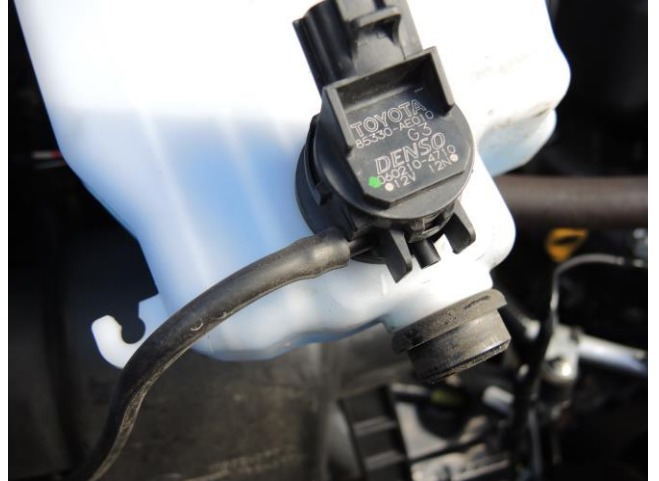
Plug hose to prevent loss of fluid ( step 3B )
