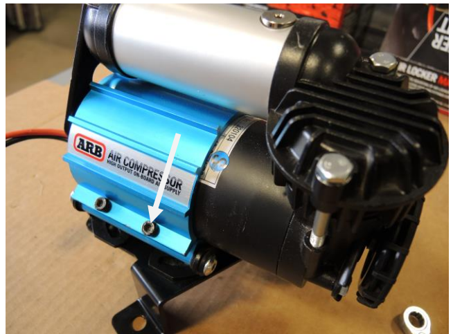
Slide compressor forward ( step 7 )
