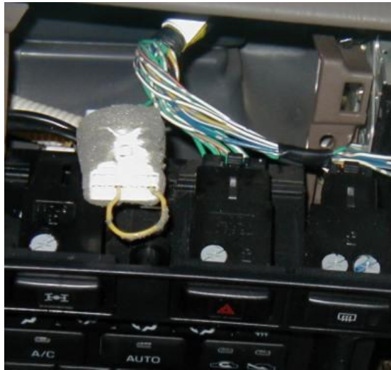
Diff lock switch harness with terminating plug installed (Step 2)
