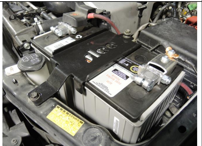
Install battery and tie down bracket (Step 6)
