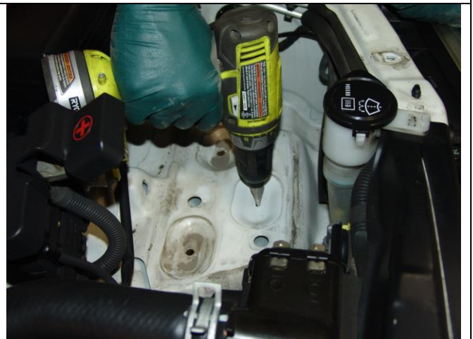
Remove hardware on reservoir ( Step 2 )
