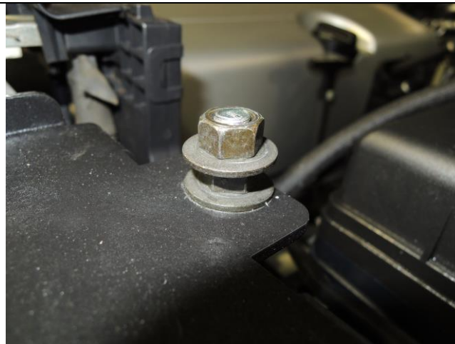
Double Nut on J-Bolt ( Step 6B )
